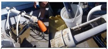
**Figure 2.** Sonde in protective shroud attached to a frame and concrete anchor for marine bottom deployments (left), with focus on sensor end (right).
