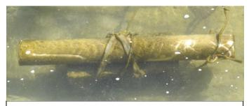
**Figure 1**. Algae and other fouling materials adhering to shroud and monitor. To protect monitors and reduce the need for abrasive cleaning, a shroud can be used to cover
